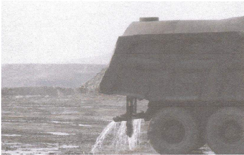
Fig. 2b: Sprinkling of water in the dump area
