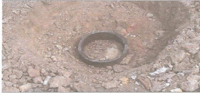
Fig. 4: Collection of field sample for testing of Physico mechanical Properties of dump material
